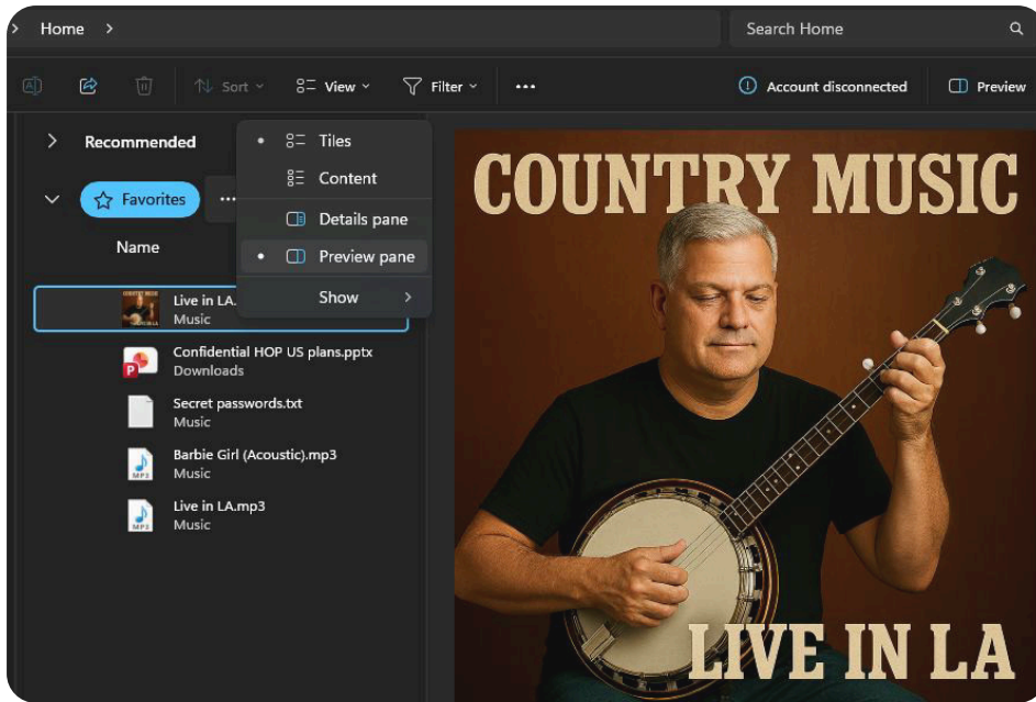
Figure 15: The Preview Pane was a continuous source of critical vulnerabilities in 2025, allowing attackers to exploit file previews to gain code execution without the user opening the file.
